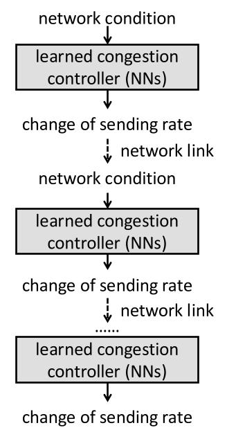
• When the network condition changes from bad to good, the sender eventually increases packet sending rates.
