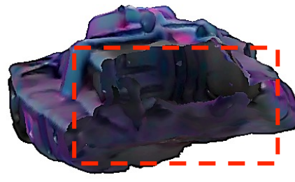
Missing Interior Mesh
