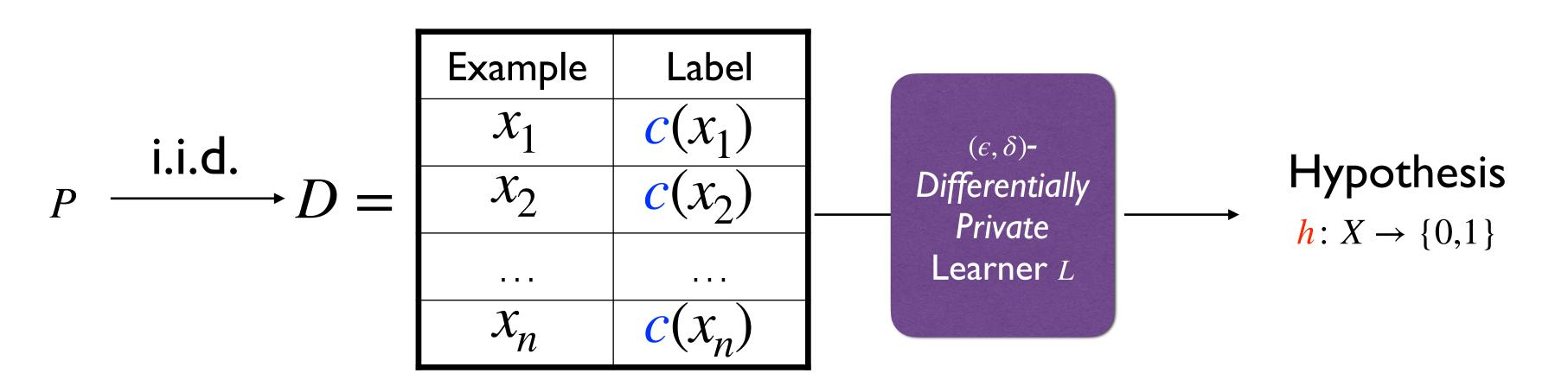
Definition: An algorithm L is  $(\epsilon, \delta)$ -differentially private if for all pairs of D, D' that differ by one example and every  $S \subseteq \text{Range}(L)$
