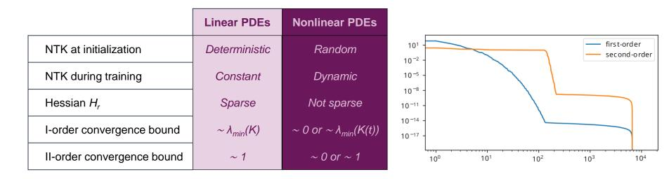
While ensuring **fast convergence**, second-order methods mitigate the issue of **spectral bias** when training PINNs on PDEs containing high-frequency components.
