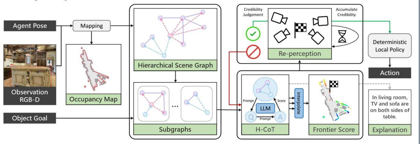
■ We densely connect the newly detected nodes to previous nodes in an incremental manner. We further prune the dense connected edges to make the 3D scene graph more precise.
