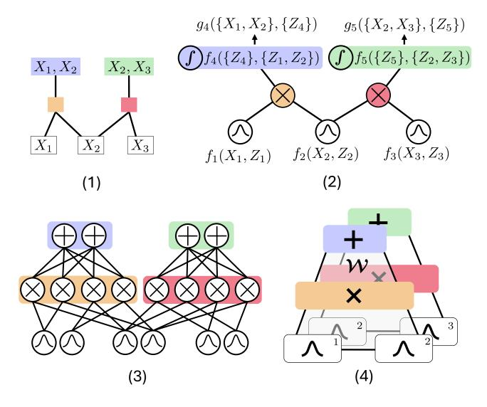
We present a pipeline that from arbitrary variable decompositions (1) builds DAG-shaped PICs (2), that we train by materializing them as tensorized circuits (aka *tensor networks*) called Quadrature-PCs (QPCs) (3), which we also fold to allow fast inference (4).
