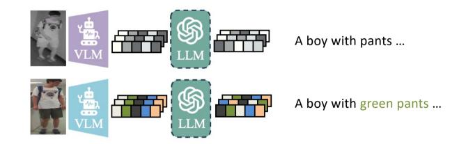
MSC introduces fine-tuned VLMs as captioners to **automatically** generate **heterogeneous** text from visible and infrared images, and utilizes LLM rephrasing for text augmentation.
