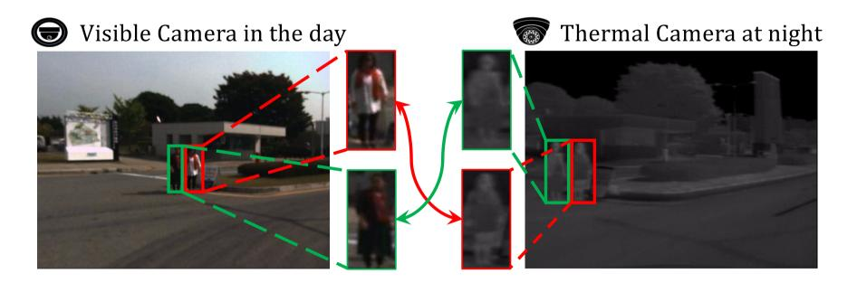
Learn a cross-modality ReID model on a set of visible-infrared images with identity labels
