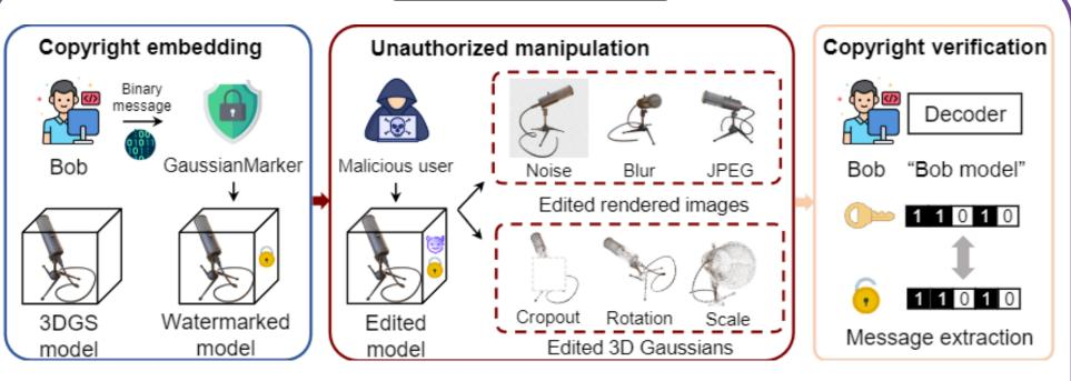
Users can apply GaussianMarker to protect their 3DGS models. If unauthorized users maliciously edit the watermarked 3DGS model, the model owners can reliably retrieve the copyright message from the altered 3D Gaussian parameters or rendered 2D images to verify ownership.
