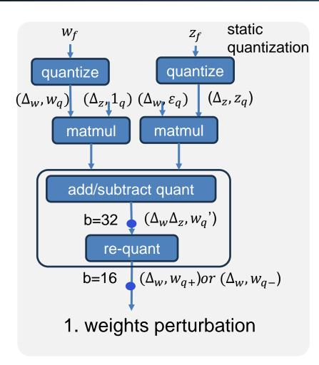
**Quantized Perturbation:** the quantized weights perturbation can be defined and calculated as:
