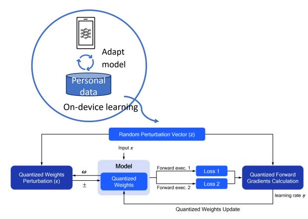
Model adaptation through fixed-point forward-forward (FF) gradient learning. Forward gradients are estimated through **forward calls only**, without the need of backpropagation.
