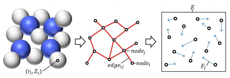
(a) [Input] An atomic structure (b) [Preprocessed] Graph (Optional) (c) [Output] Energy and Forces
