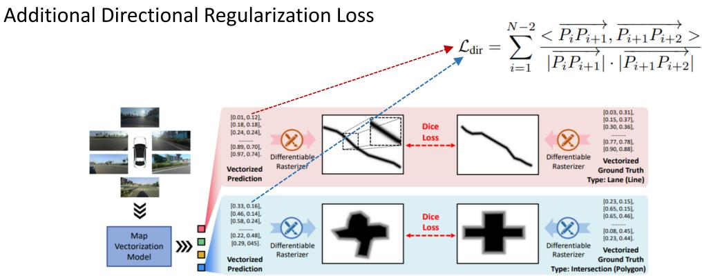
Figure : The learning pipeline of MapVR. MapVR utilizes a base model for vectorized map generation, followed by a customized differentiable rasterizer to produce HD maps, on which fine-grained, geometry-aware supervision is applied to enhance the precision of vectorized elements.
