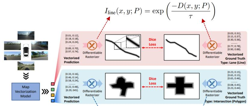
Figure : The learning pipeline of MapVR. MapVR utilizes a base model for vectorized map generation, followed by a customized differentiable rasterizer to produce HD maps, on which finegrained, geometry-aware supervision is applied to enhance the precision of vectorized elements.
