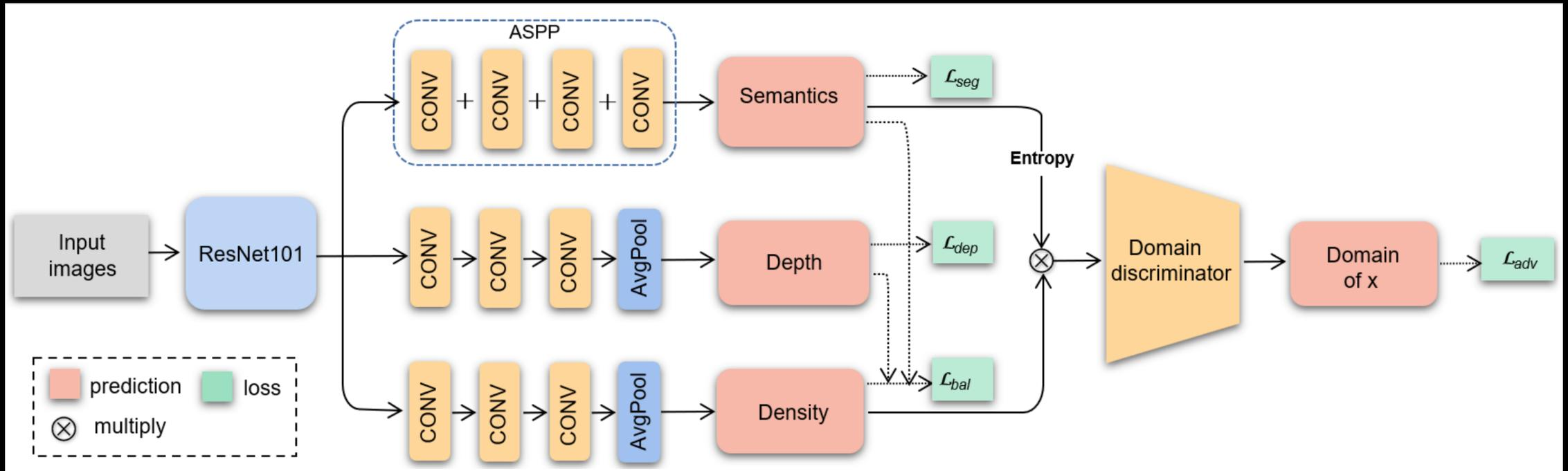
We use standard multi-task learning framework to obtain three sub-tasks, i.e. semantic segmentation, depth regression, and **depth distribution density estimation**.
